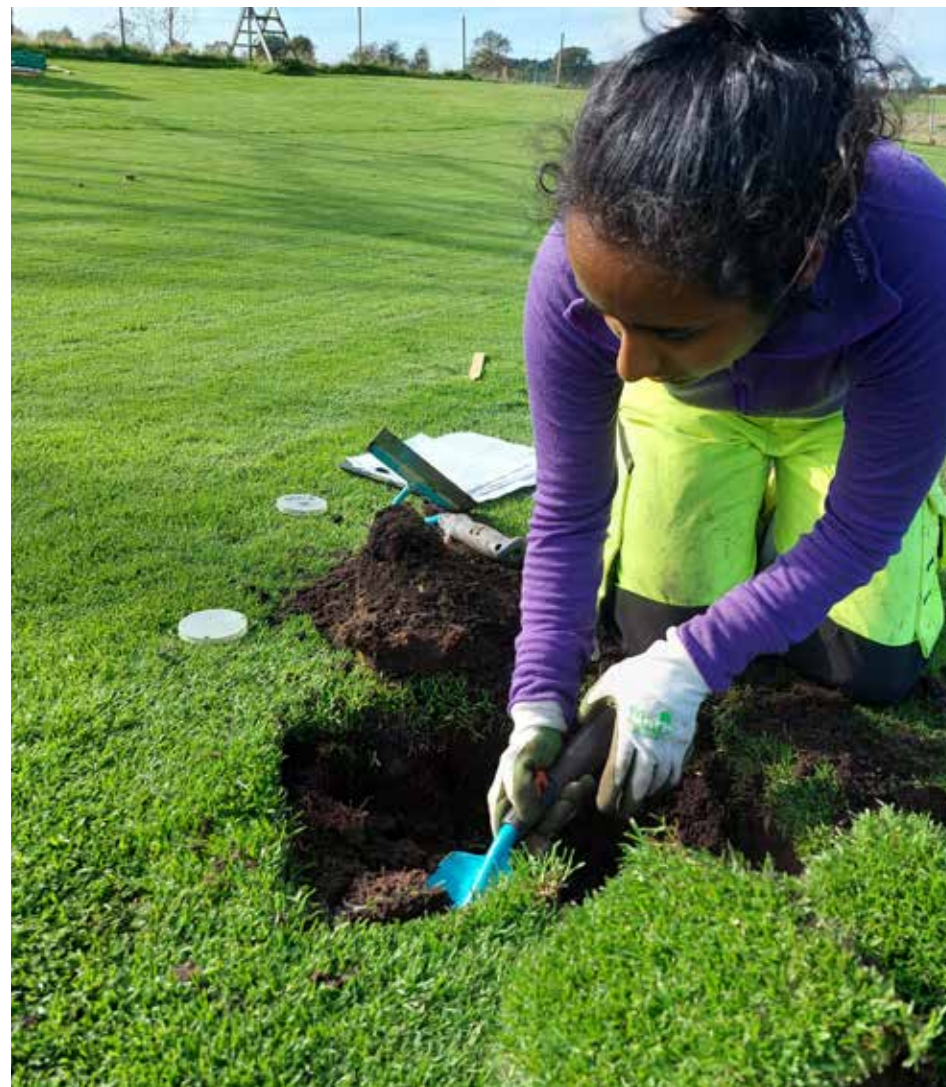
Monica Jayesingha taking undisturbed soil samples for soil density analysis at Berheim GC in September 2023. Photo: Anne F. Borchert.
